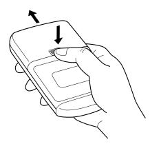
Replacing the battery Put the batteries in the case observing the polarities as illustrated.
